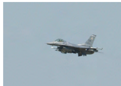
Wake turbulence result when higher pressure air flows around the wing tip toward the relatively low pressure air above the wing. Wake turbulence from an F-16 aircraft is approximately 7 mph for a 300-foot overflight.
