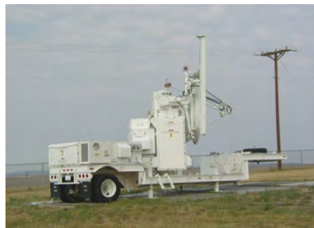
The signals from this threat emitter system simulate an integrated air defense system typical of defenses encountered in combat.
